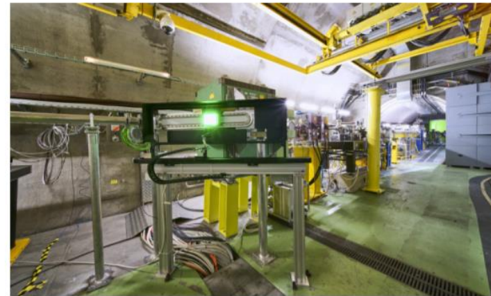
The final part of the AWAKE experimental facility, with the accelerating plasma cell and the scintillating screen used to detect the accelerated electrons and infer their energy. (Image: Maximilien Brice, Julien Ordan/CERN)
